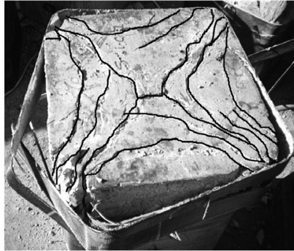
(b) Dilated square column confined with carbon/epoxy jacket [19]
